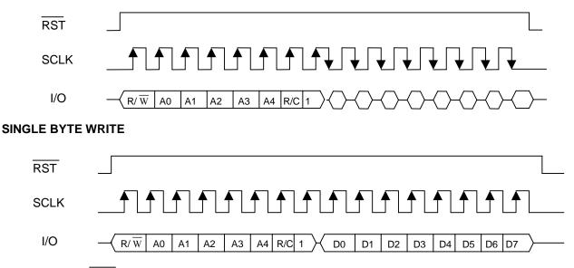
In burst mode,  $\overline{RST}$  is kept high and additional SCLK cycles are sent until the end of the burst.
